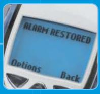
The system can be reset remotely using a touchtone telephone.
