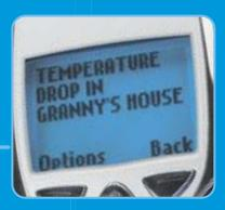
Users can define the message that each of four separate triggers send to telephones.
